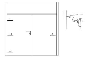
**6.** Using long countersunk frame fixings, first fix as shown, with 3 fixings in the active leaf jamb and 1 in the fixed leaf jamb.
