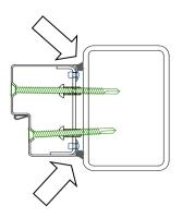
**12.** Apply mastic or flashings to seal frame to building. Fire rated doorsets must be sealed as shown, all round the frame, using either:
