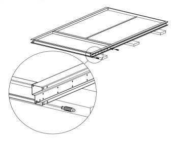
**2.** Slide transom between jambs then attach to frame with taptite screws. Tighten all screws.
