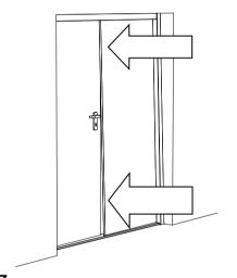
7. Open the doors, discard the transit packings, then close and lock the fixed leaf. With the active leaf nearly closed, check the alignment between the active leaf lock edge, and the slam bar frame seal, at both the top and bottom of the doors.
