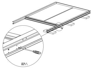
**1.** Assemble the doorset in front of the opening.
