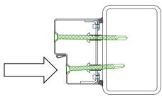
**9.** Open the doors fully, then tighten the 2nd set of frame adjusters in the reveals.
