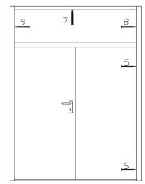
**8.** Close the active leaf again, then fit the last 2 fixings into face 5 of the fixed leaf jamb and fixings into transom and head.
