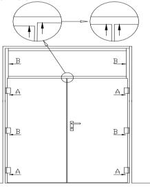
**3.** Align and grip the doorset in the opening, using the frame adjusting screws A in the corners, then the middle adjusters B.
